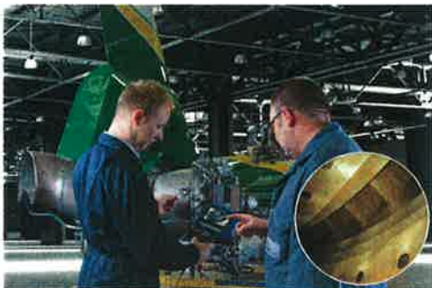
Inspecting a helicopter turbine with the MoVeo videoscope
